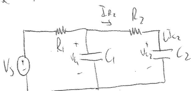
$$V_s = V_{R_1} + V_{C_1}$$
