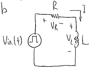
$$V_{in} = V_R + V_L \rightarrow V_{in} = RI + L \frac{dI}{dt}$$
