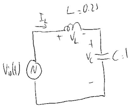
$$V_{in} = V_L + V_C \quad I_L = I_C = C \frac{dV_C}{dt} \quad \boxed{\frac{dV_C}{dt} = \frac{I_L}{1} = I_L}$$
