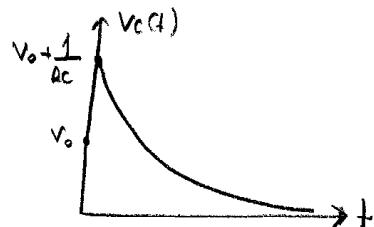
\* The zero state impulse response is the time-derivative of zero state unit step response -
