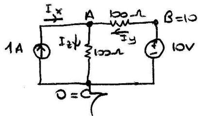
$$\begin{aligned} I_x + I_y &= I_b \\ \frac{I}{100} + \frac{B-A}{100} &= \frac{A-C}{100} \\ 100 + B - A &= A - C \\ 100 + B + C &= 2A \end{aligned}$$
