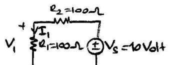
$$V_1 = V_s \frac{R_1}{R_1 + R_2} = 10 \frac{100}{100 + 100} = 5V$$
