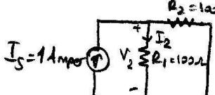
$$I_2 = I_s \frac{R_2}{R_1 + R_2} = 1 \frac{100}{100+100} = 0.5 \text{ Amper}$$
