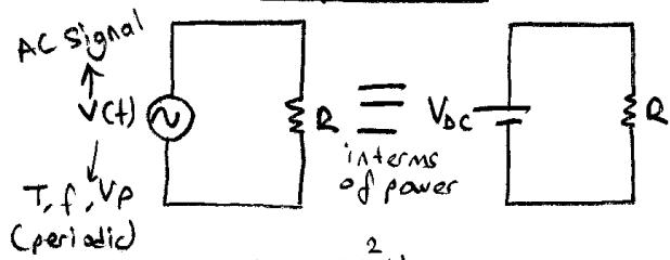
what is the value for  $V_{DC}$  such that ( $V_{DC}$  is a DC Value) both circuits produce some amount of energy in the same period of time?
