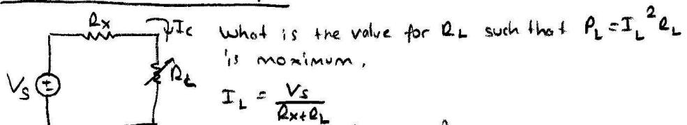
What is the value for  $R_L$  such that  $P_L = I_L^2 R_L$  is maximum.
